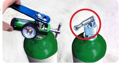
Once the regulator is on, use the wrench to open the tank (turn to the left to open). Some tanks have a wrench built in. You can twist that to the left to open the tank.
