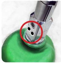
The "teeth" will fit into the matching two holes on the neck of the oxygen tank.
